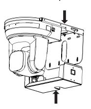
8. Tighten the screws on either side to secure the metal plate cover
