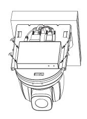
7.Pack the cables neatly and latch the metal plate cover
